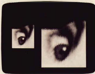
Cameras that have "random sync" generate vertical streaks in an image. Note the shifts across the center of the pupil.
